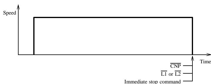
Diagram 3-25 Example of Constant speed origin search operation
