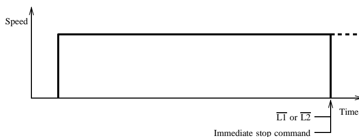
Diagram 3-19 Example of Continuous Constant Speed Operation
